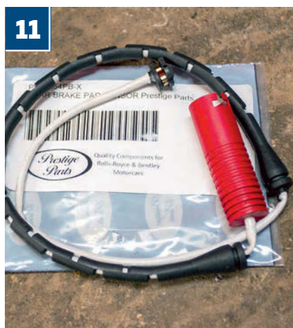
11 Pad level warning sensors are easy to forget when ordering new braking components; this is the rear sensor (only one required per car)
