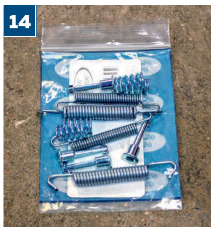
14 ... and this is the corresponding handbrake shoe fitting kit, including pins and springs – with all parts being from IntroCar's Prestige Parts range
