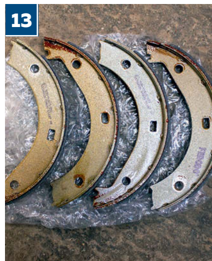
13 Next up is a new set of handbrake shoes...
