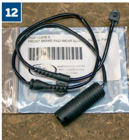
12 This is the front pad wear sensor, again with only one required per car; you'll note how sensors are colour coded to ensure avoidance of incorrect fitment
